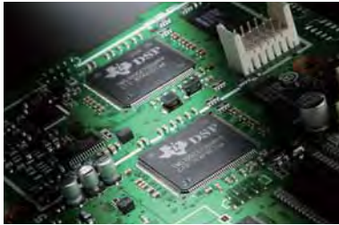
DSP unit for Transmit and Receive TMS320C6726B (Top in photo) Internal clock speed: 266MHz 32-bit floating point DSP Maximum performance =1600MFLOPS DSP unit for Spectrum scope TMS320C6720 (Bottom in photo) Internal clock speed: 200MHz 32-bit floating point DSP Maximum performance =1200MFLOPS
